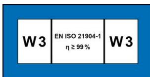
Products with W3 certification according to requirements for W3/IFA certified welding fume separation class. (See "Technical data" chapter)
